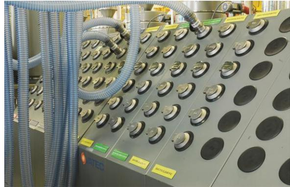
*A single operator using a manifold like this one directs the right materials to the right machines, making changeovers both faster and more secure.*
