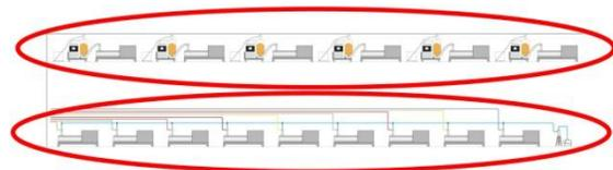
*Removing individual drying and handling equipment from six injection molding machines allowed three more machines in the same floor space.*
